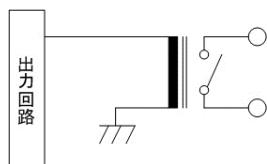
ICL-13A-AA/MM [無接点電圧出力(SSR駆動用)]
