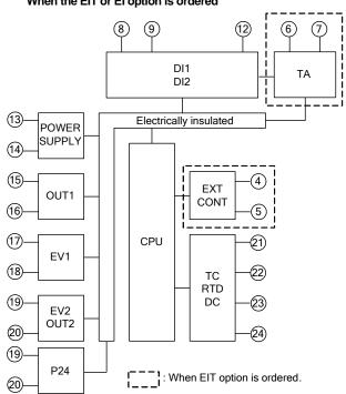
If OUT1 is a non-contact voltage output or direct current output, and if OUT2 is a non-contact voltage output or direct current output, OUT1 is not electrically insulated from OUT2.
