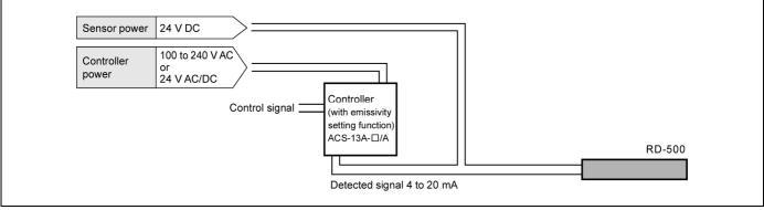
Close focus type (RD-5CF-H0) is 4-wire type, but 2 wires are not used.)
