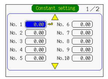
Move the cursor to the relevant constant No. and press the ENT key to display the following constant setting screen. Enter the decimal point position and constant using the cursor key and the ENT key.
