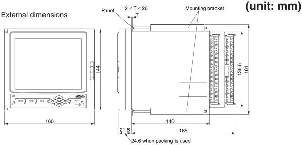
Note) If other instruments are placed under the recorder unit, provide a space of 100 mm or more from the instrument or floor.
