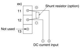
Example 1) For 4 to 20mA and 10 to 50mA input,  $10\Omega\pm0.1\%$  shunt resistance is used.
