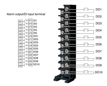
Note: If lamps are provided on the outside, set a resistor to prevent rush current. When relays or solenoids are used, set elements for contact protection (diodes or surge killers, etc).
