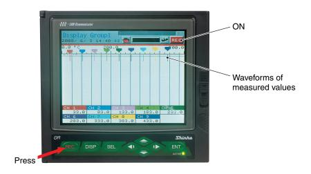
2) When the password for stopping and starting the record operation is set, the password setting screen is displayed as follows. Therefore, make a setting of the password. When the password is correct, the recording is started.
