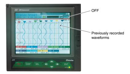
3) When the password for stopping and starting the record operation is set, the password setting screen is displayed as follows. Therefore, make a setting of the password. When the password is correct, the recording stop confirmation screen is displayed.
