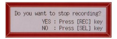
2) After the stop of the recording, the REC lamp comes off. The trend display on the data display unit stops. In this case, even if there is some data that are not yet written in the memory card, the unit writes them in the card until the recording is finished.
