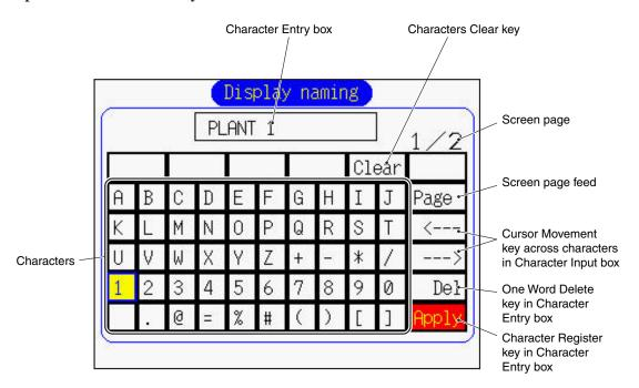
Note: To make the set characters valid, select the "Apply" key and press the ENT key. The set characters will not be valid without pressing the ENT key.
