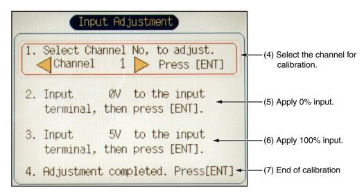
Select the channel for calibration by using the cursor key and press the (ENT) key.
