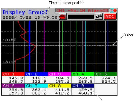
Measured value at cursor position of each channnel(Min and Max values)
