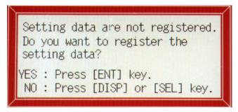
(5) When the password for parameter setting or compact flash operation is set, the following password setting screen may be displayed for displaying each parameter setting screen. Therefore, make a setting of the password. When the password is correct, the setting screen is displayed.
