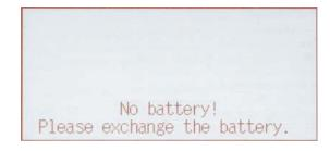
(5) When power is turned OFF because of power failure during recording
