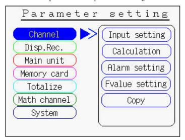
Note: After setting the parameters, click "Main Unit" → "Register data" in order to save the set information to a flash memory. To refresh parameter set values, press (DSP) key. So, the following message appears, prompting you to select the option. Press the (ENT) key twice. Now, the parameter has been refreshed.
