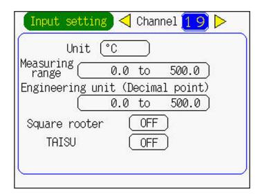
For operation procedure, refer to "8.4 Setting for input types, skip, scaling, units and square rooter".
