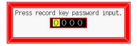
3) If the CF card is not inserted, the following message appears. Press the (REC) or the (ENT) key to start recording. Press the (SEL) key not to start recording.
