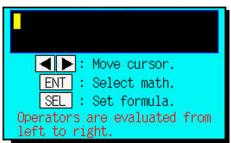
Press the ENT key on the formula setting screen to display the Menu screen. Move the cursor to the target formula and press the ENT key.
