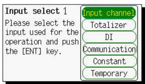
• Channel input : Enter the channel No. to be used.
