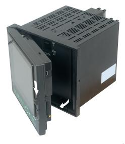
Step 2) Insert the memory card into the slot at the right side of the panel unit as shown in Photo.
