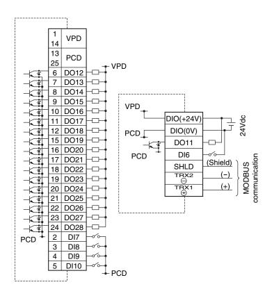
Note 1: The DI (external control unit) is not insulated. Connect a relay externally to use the unit.
