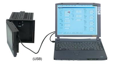
The loader cable should be connected to the USB port of PC.
