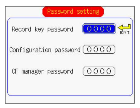
Move the cursor to the parameter to be changed. Pressing the key displays the "Parameter Setting" screen. Set the password using the cursor, and press the key. Set "0000" to reset the password setting.
