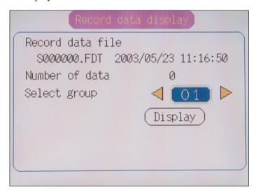
(2) Select the screen group No. to be displayed using the cursor key and press the wey, and the cursor moves to the "Display." Then press the wey key to display the historical trend screen of the group No. selected.
