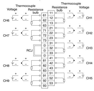
Note) For current input, connect optional shunt resitors to the voltage input terminals.
