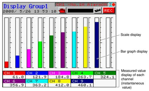
2. The measured data is displayed in analog meters.
