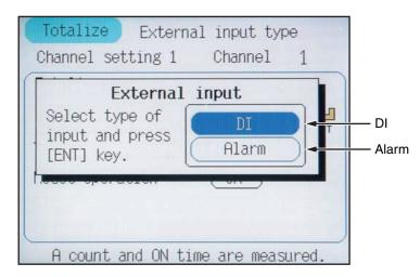
Move the cursor to DI and press the (ENT) key. On the External type screen that appears, select DI No. with which totalize start/stop is controlled using the cursors on both sides.
