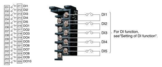
Note 1) DI (external control) unit is not insulated and should be used with a relay connected to the outside.
