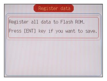
To save set values to the internal memory, press the (ENT) key.
