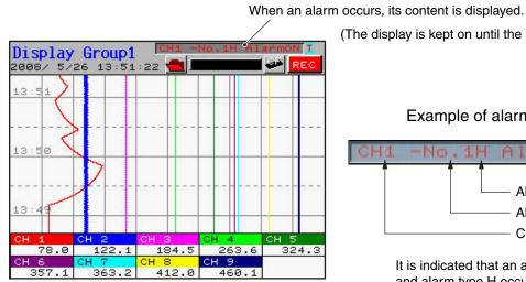
(The display is kept on until the alarm is reset.)
