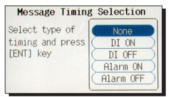
Select any item by the cursor key and press the ENT key. After selection, the "Message Timing" screen appears as shown below. Set the "Channel" and "Alarm No." by the cursor key. After setting them, press the ENT key for confirmation.
