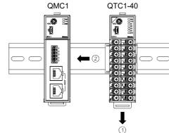
③ Raise the lock lever of the QTC1-40. Make sure it is fixed to the DIN rail.
