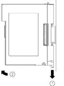
Mounting multiple modules to the DIN rail
