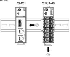
3 Raise the lock lever of the QTC1-40. Make sure it is fixed to the DIN rail.
