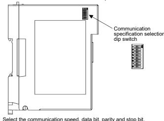
Select the communication speed, data bit, parity and stop bit
