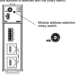
Use a small flat blade screwdriver to select the module address The module address of QMC1 differs depending on the model name.
