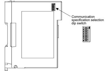
Select the communication speed, data bit, parity and stop bit. All are off when shipped from the factory.
