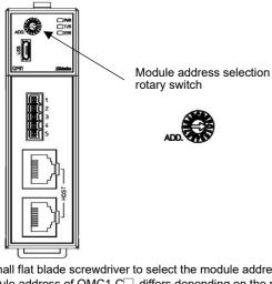
Use a small flat blade screwdriver to select the module address The module address of QMC1-C differs depending on the model name
