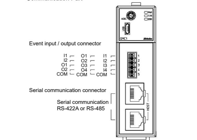
(1) Pin arrangement of event input / output connector
