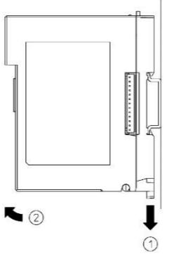
Mounting multiple modules to the DIN rail
