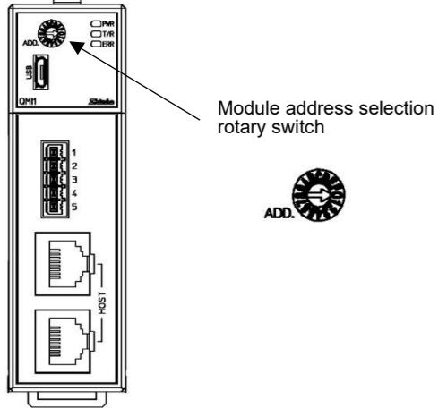
Use a small flat blade screwdriver to select the module address. The module address of QMC1-C□ differs depending on the model name.
