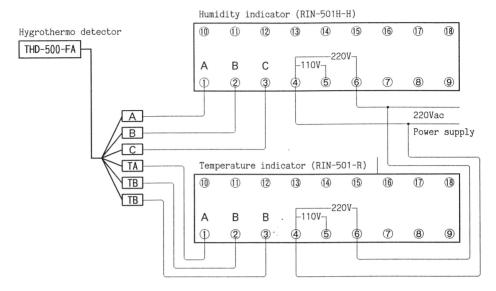
Notes: • Power source (5Vdc) for humidity sensor is built-in the Humidity indicator RIN-501H-H.
