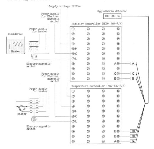
Notes: • Power source (5Vdc) for humidity sensor is built-in the Humidity controller MCD-110H-R/H.
