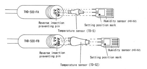
Notes: • Do not mount the sensor excepting TD-S or TD-S2 for temperature and HD-S2 for humidity.
