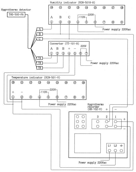
Notes: • Power source (5Vdc) for humidity sensor is built-in the Humidity indicator RIN-501H-H.
