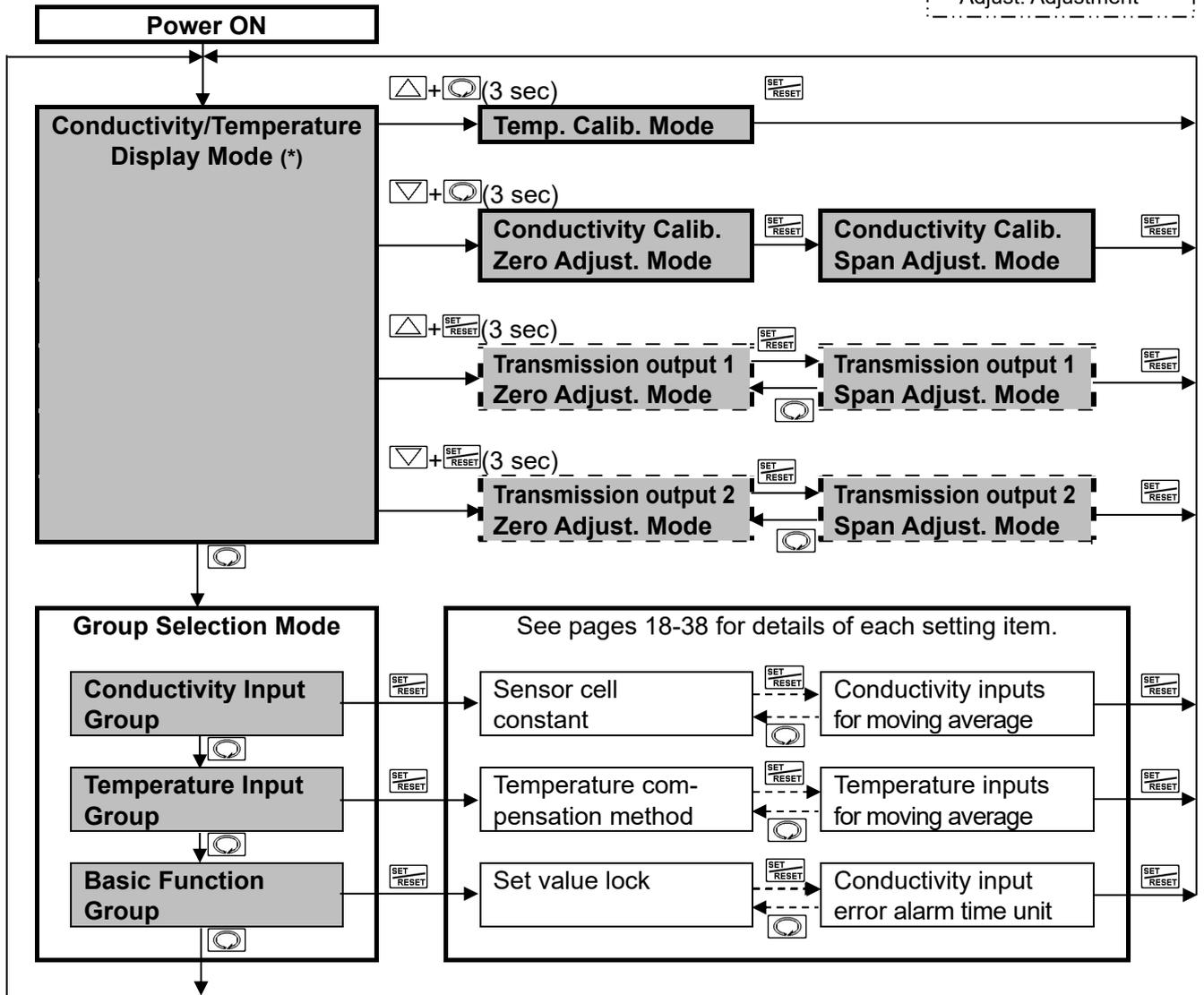
(\*) Indicates the item selected in [Display selection (p.34)] in Conductivity/Temperature Display Mode.
