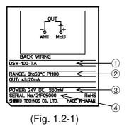
Model label is attached to the inside of the case.
