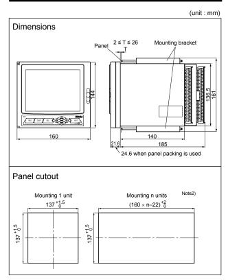
Note1) If other instruments are placed under the recorder unit, provide a space of 100 mm or more from the instrument or floor.
