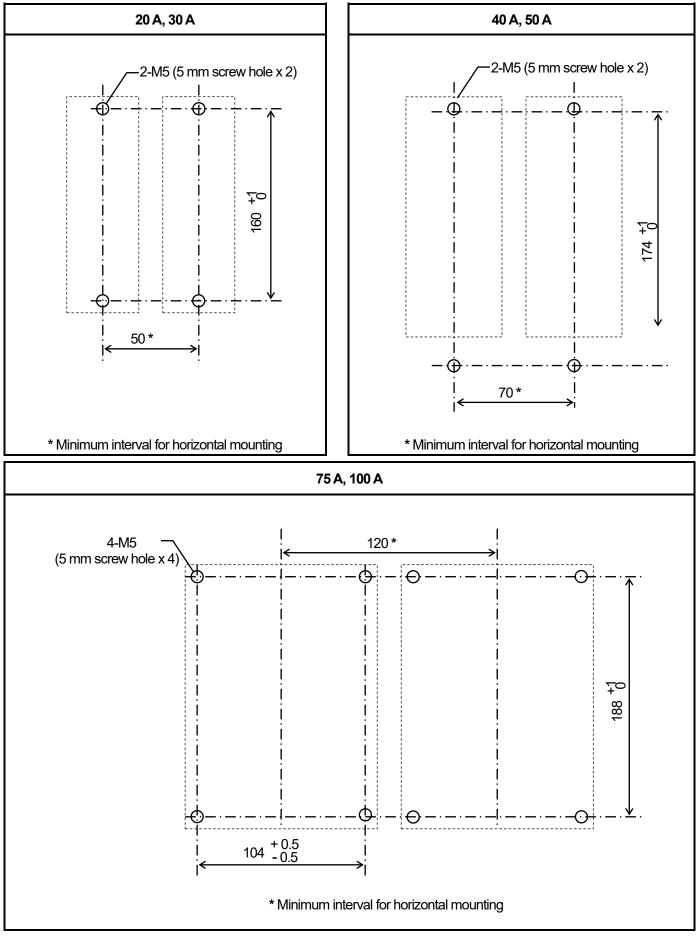
Note: Keep space for heat radiation of more than 200 mm above and below this unit.
