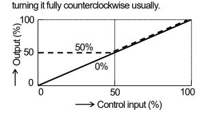
The above figure shows the lower limit setting when the gradient is set to 100%.
