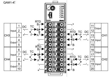
For DC current input (with an external receiving resistor), connect a receiving resistor [option 50 Ω (RES-S01-050)] between each input terminal (+ and -).
