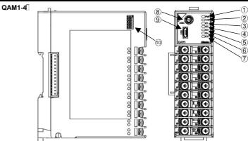
2. Overview This instrument is a 4 points Analog I/O Module.
