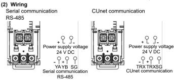
For CUnet communication, install a terminator [ optional 100  $\Omega$ (RES-S07-100)] on the last module of the communication line.
