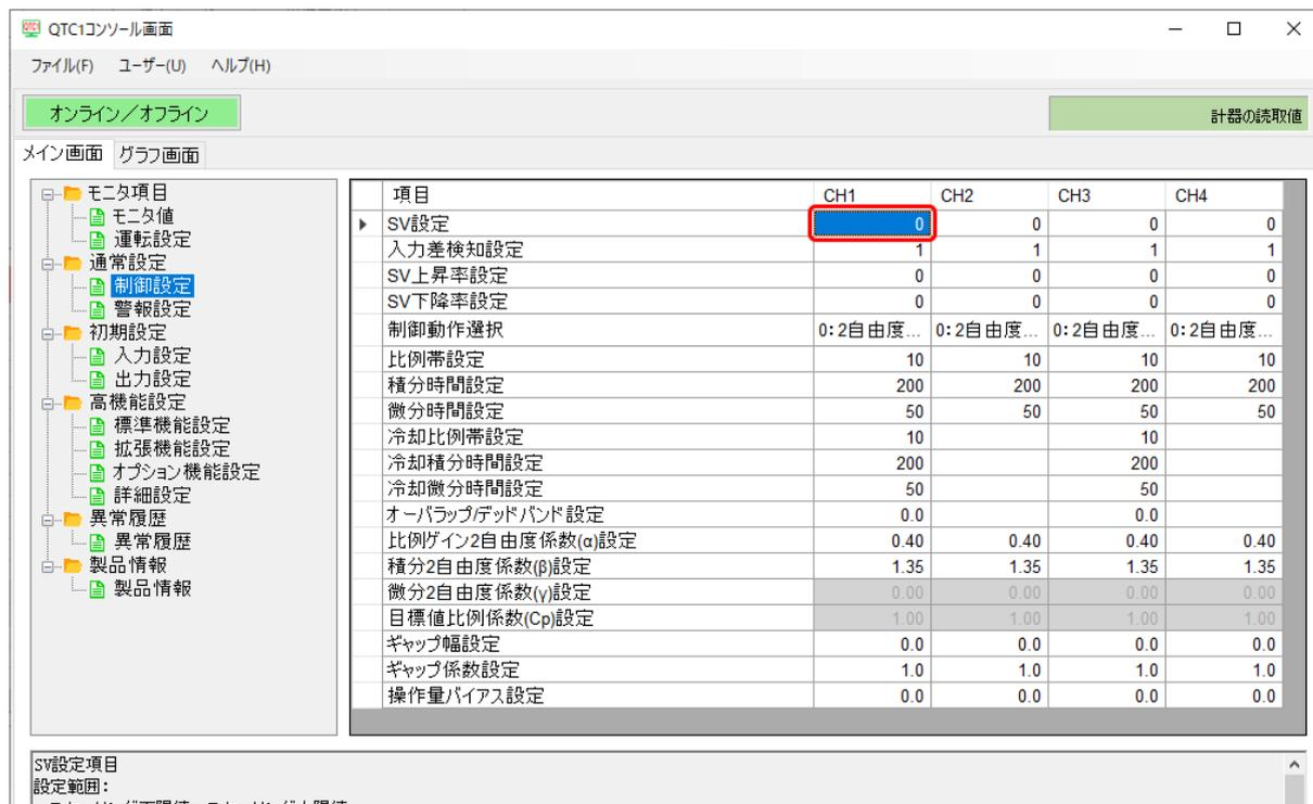
The screenshot shows the QTC1 console software interface. On the left is a tree view of settings categories, with '制御設定' (Control Settings) selected. The main area is a table with columns for '項目' (Item) and channels 'CH1', 'CH2', 'CH3', and 'CH4'. The 'SV設定' (SV Setting) row for CH1 is highlighted with a red box, showing a value of '0'. Below the table, the 'SV設定項目' (SV Setting Item) and its '設定範囲' (Setting Range) are displayed as 'スケール1/2下限值~スケール1/2上限値'.
